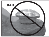
OVAL NECK OF BOLT NOT SEATED PROPERLY
