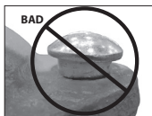
OVAL NECK OF BOLT NOT SEATED PROPERLY
