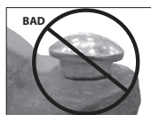
OVAL NECK OF BOLT NOT SEATED PROPERLY
