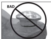
OVAL NECK OF BOLT NOT SEATED PROPERLY
