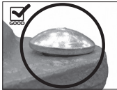
OVAL NECK OF BOLT SEATED PROPERLY
