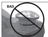
OVAL NECK OF BOLT NOT SEATED PROPERLY
