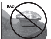
OVAL NECK OF BOLT NOT SEATED PROPERLY
