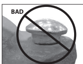
OVAL NECK OF BOLT NOT SEATED PROPERLY
