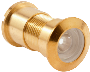
Qty: 1 Solid brass end caps, diecast housing, glass lens, 130°, fits 1-3/4 in. to 2-3/8 in. thick doors. U 9896 (Brass) U 10314 (Satin nickel finish)
