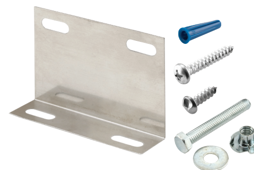
Qty: 1 set, with fasteners. Anchoring kit, for any post thickness, 3 in. to 5 in. long posts require one kit, 6 in. to 17 in. long posts require two kits, 18 in. and longer posts require 3 kits. 658-9219
