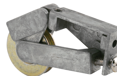
Qty: 1 Diecast housing assembly, end adjustable, 1-1/4 in. O.D. steel ball bearing roller, center grooved.
