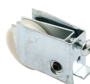
Qty: 1 Steel housing assembly, end adjustable, 1-1/2 in. O.D. plastic ball bearing roller, center grooved.
