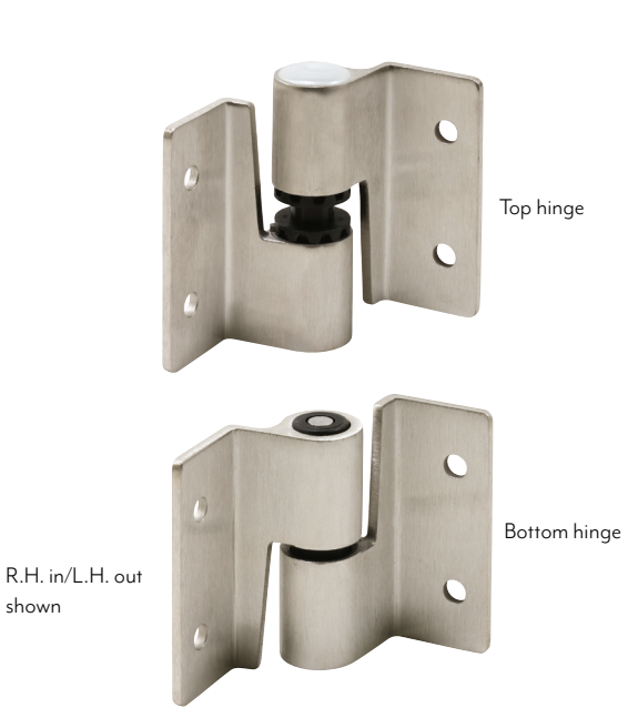
Qty: 1 set, with fasteners. Top and bottom, surface mounted, 1-1/2 in. hole spacing. 658-8621 (Satin cast stainless steel – R.H. in/L.H. out) 658-8056 (Satin cast stainless steel – L.H. in/R.H. out)
