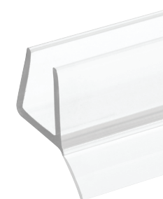
Qty: 1 Clear vinyl, 36 in., bottom mount, slip-on fit. M 6262 (Fits 1/4 in glass) M 6264 (Fits 3/8 in glass) M 6268 (Fits 1/2 in glass)
