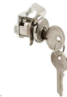
Qty: 1 set, 2 keys. Diecast cylinder, 5-pin tumbler, spring steel locking clip, steel cam. S 4130 (Nickel)
