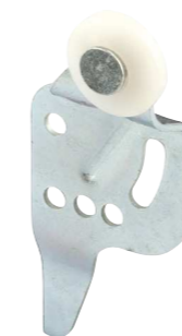
Qty: 2, with fasteners. Steel bracket, 5/8 in. offset, top hung, adjustable, 7/8 in. O.D. plastic roller, flat edge, for 3/4 in. to 1-3/8 in. thick doors.
