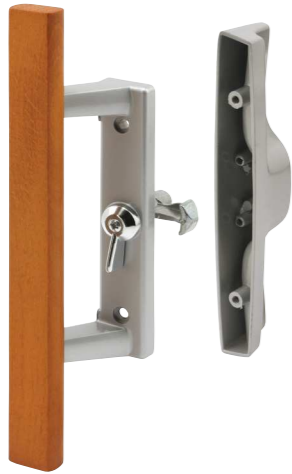
Qty: 1 set, with fasteners. Diecast inside pull with wood handle, diecast outside handle, 3-15/16 in. hole spacing, hook style, internal lock, reversible, for 1-3/4 in. thick doors.
