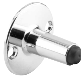
Qty: 1, with fasteners. Door stop, 1-19/32 in. hole spacing, 2 in. projection.
