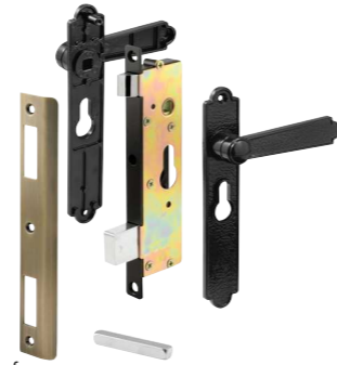
Qty: 1 set, with fasteners. Diecast handles with 6-9/16 in. hole spacing, diecast mortise lock with 6-3/4 in. hole spacing, 1-1/4 in. backset.
