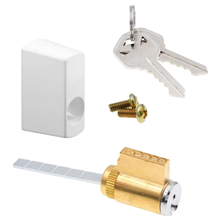
Qty: 1 set, 2 keys, with fasteners. Diecast housing, solid brass cylinder, hardened break-away tailpiece, 5 pin tumbler, 1-3/4 in. hole spacing. E2145 (White)
