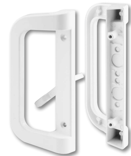
Qty: 1 set, with fasteners. Diecast handles with thumbturn, 3-15/16 in. hole spacing, hook style, mortise latch, non-handed.
