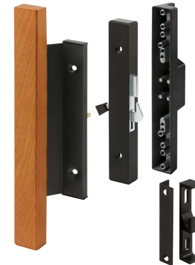
Qty: 1 set, with fasteners. Extruded aluminum inside pull with wood handle, diecast outside handle, 4-15/16 in. hole spacing, hook style latch, surface mounted, reversible. C1105 (Black)
