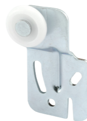
Steel bracket, top hung, adjustable, 7/8 in. O.D. plastic roller, round edge, for 3/4 in. to 1-3/8 in. thick doors.
