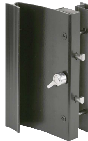
Qty: 1 set, with fasteners. Extruded aluminum handles, 3-7/8 in. hole spacing, hook style latch, surface mounted, for Ador Hilite® doors. C1014 (Aluminum) C1015 (Black)
