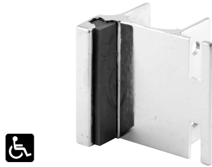
Qty: 1, with fasteners. Inswing for throw latch (emergency entrance), for 1-1/4 in. thick round edge posts, 1-1/2 in. hole spacing. 656-6521 (Chrome plated zamak)
