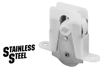
Qty: 2, with fasteners. Stainless steel inner housing, plastic outer housing, adjustable, 1 in. O.D. stainless steel ball bearing roller, center grooved.
