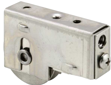
Qty: 1 Stainless steel housing assembly, end adjustable, 1-1/2 in. O.D. stainless steel ball bearing roller, center grooved.
