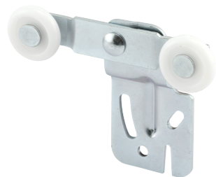
Steel bracket, top hung, adjustable, tandem 7/8 in. O.D. plastic rollers, round edge, for 3/4 in. to 1-3/8 in. thick doors.
