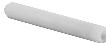
Qty: 1 Knurled plastic, 1/4-20 thread, 3/8 in. O.D., used by Sanymetal.
