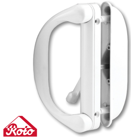
Qty: 1 set, with fasteners. Diecast handles with thumbturn, 4-15/16 in. hole spacing, hook style, mortise latch, 7/32 in. square drive, non-handed. C1275 (White)
