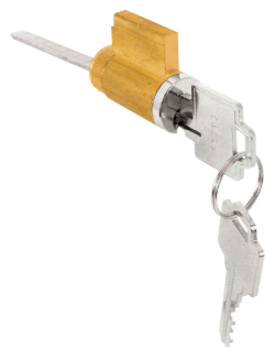
Qty: 1 lock, 2 keys. Solid brass cylinder, hardened break-away tailpiece, 5 pin tumbler, keyway is compatible to Weiser®, Kwikset®, and Weslock®.
