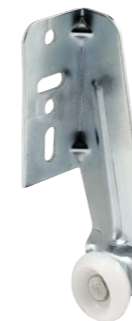
Qty: 2, with fasteners. Steel bracket, convex plastic roller, 3/4 in. O.D., mounts on rear of drawer.
