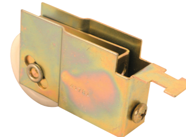
Qty: 1 Steel housing assembly, end adjustable, 1-1/2 in. O.D. plastic ball bearing roller, center grooved.
