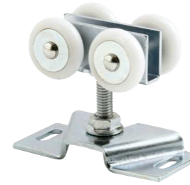
Qty: 2, with fasteners. Steel bracket, adjustable, (4) 7/8 in. O.D. plastic rollers, round edge, for 1-3/8 in. thick doors.
