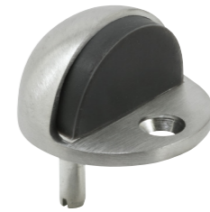
Qty: 1, with fasteners. Cast brass housing, rubber bumper, 15/16 in. hole spacing, floor mounted, meets ANSI standards.
