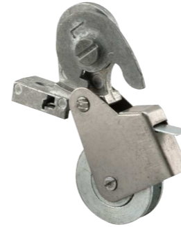
Qty: 1 left and 1 right. Stamped steel housing, diecast mounting bracket, adjustable, 1 in. O.D. steel ball bearing roller, center grooved.
