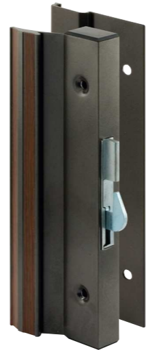
Qty: 1 set, with fasteners. Extruded aluminum handles, 4-15/16 in. hole spacing, hook style latch, surface mounted, reversible.
