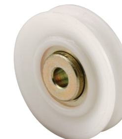
Qty: 2 Plastic ball bearing roller, 1-11/16 in. O.D., 1/4 in. I.D. axle hole, center grooved. D 1716 (Steel race)
