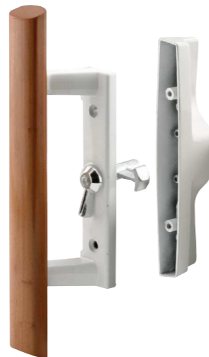
Qty: 1 set, 2 keys (if keyed), with fasteners. Diecast inside pull with wood handle, diecast outside handle, 3-1/2 in. hole spacing, hook style, internal lock, reversible, for 1 in. thick doors.
