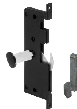
Qty: 1, with fasteners. Plastic latch, steel hook and keeper, 3-7/8 in. hole spacing, non-handed.
