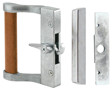
Qty: 1 set, with fasteners. Diecast inside pull with wood handle, diecast outside handle, 3 in. hole spacing, hook style latch, surface mounted, fits Fullview® doors. C1023 (Aluminum)
