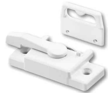
Qty: 1 set, with fasteners. Diecast with alignment lugs, 2-1/4 in. hole spacing, cam action. F2767 (White)
