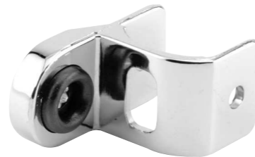
Qty: 1, with fasteners. In/outswing for concealed latch with round bolt, for 1-1/4 in. thick round edge posts. 656-6530 (Chrome plated zamak)
