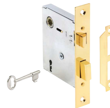
Qty: 1 set, 2 keys, with fasteners. Brass plated steel, keyed, spindle hole accepts 1/4 in. to 5/16 in. square spindles, 2-3/8 in. backset.
