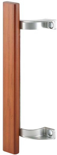
Qty: 1, with fasteners. Diecast mounting base with wood handle, 6-1/2 in. and 6-5/8 in. hole spacing, mounting holes are slotted, surface mounted.
