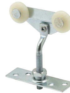
Qty: 1, with fasteners. Steel bracket, top hung, adjustable, tandem 3/4 in. O.D. plastic rollers, round edge, for 3/4 in. to 1-3/8 in. thick doors.
