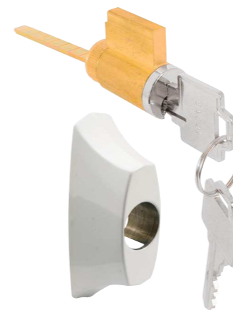
Qty: 1 set, 2 keys, with fasteners. Diecast housing, solid brass cylinder, hardened break-away tailpiece, 5 pin tumbler, 2-1/2 in. hole spacing. E2144 (White)
