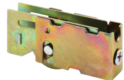
Qty: 1 Steel housing assembly, end adjustable, 1 in. O.D. steel ball bearing roller, center grooved.
