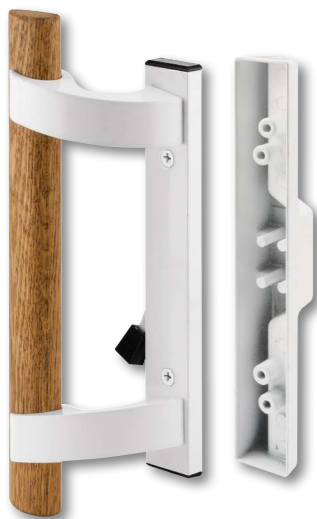
Qty: 1 set, with fasteners. Extruded aluminum inside pull with wood handle and thumbturn, diecast outside handle, 3-15/16 in. hole spacing, hook style, mortise latch, non-handed.
