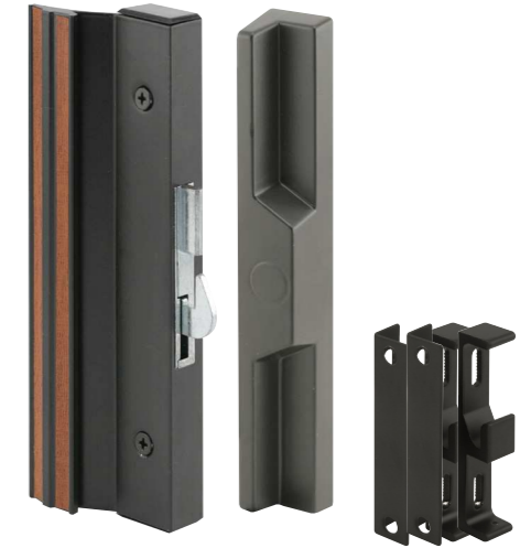
Qty: 1 set, with fasteners. Extruded aluminum inside pull, diecast outside handle, 4-15/16 in. hole spacing, hook style latch, surface mounted, reversible.
