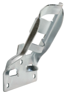
Qty: 1, with fasteners. Stamped steel, 35° projection from vertical, for poles 3/4 in. O.D. U 9379 (White) U 9378 (Zinc finish)
