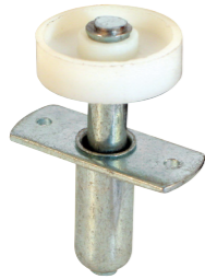
Qty: 2, with fasteners. 3/8 in. O.D. steel base, top mount, spring loaded, self-adjusting, 3/4 in. O.D. plastic roller, flat edge, for 1 in. to 1-3/8 in. thick doors.
