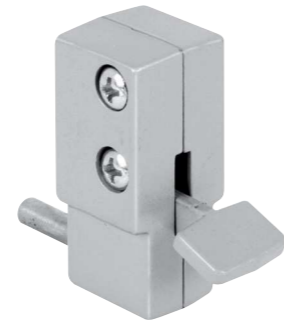
Qty: 1, with fasteners. Diecast housing, hardened steel bolt, foot operation, 5/8 in. projection, 5/8 in. hole spacing.
