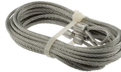
Qty: 2 Galvanized carbon steel, 8 ft. 8 in. length, with stops. GD 52183 (1/8 in. cable) GD 52263 (3/32 in. cable)
