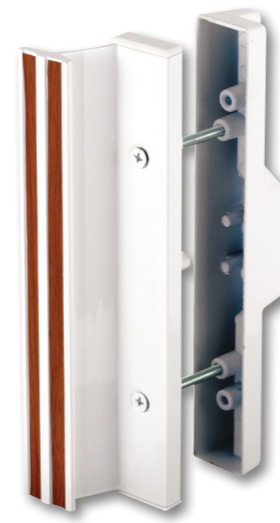
Qty: 1 set, with fasteners. Extruded aluminum inside handle and thumbturn, diecast outside handle, 3-15/16 in. hole spacing, hook style, mortise latch, non-handed.
