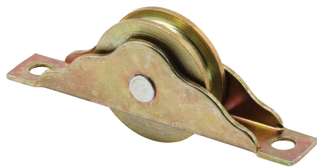
Qty: 2 Solid brass housing, fits a 2-15/16 in. x 7/16 in. mortise slot, 2-1/2 in. hole spacing, 1-3/16 in. O.D. steel ball bearing roller, center grooved.
