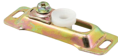
Qty: 1, with fasteners. Steel with plastic bushing, adjustable, 2-11/16 in. hole spacing, floor mounted, accepts a 1/4 in. O.D. pin.
