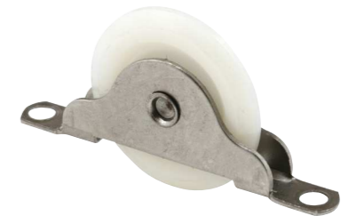
Qty: 2, with fasteners. Steel housing, fits a 2-1/4 in. x 9/32 in. mortise slot, 2 in. hole spacing, 1-3/16 in. O.D. plastic roller, round edge.
