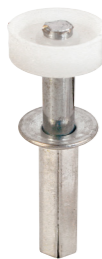
Qty: 2 7/16 in. O.D. steel base, top mount, spring loaded, self-adjusting, 7/8 in. O.D. plastic roller, flat edge, for 1 in. to 1-3/8 in. thick doors.
