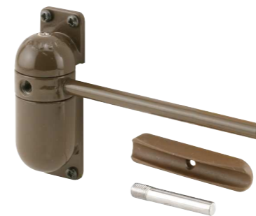
Qty: 1, with fasteners. Diecast zinc body incorporates one torsion spring, adjustable, weather resistant, non-handed, for doors and gates up to 57 lbs.
