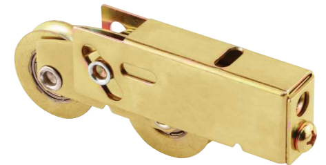
Qty: 1 Steel housing assembly, end adjustable, tandem steel ball bearing rollers, center grooved. D1979 (1 in. O.D.) D1735 (1-1/4 in. O.D.)
