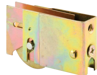
Qty: 1 Steel housing assembly, end adjustable, 1-1/2 in. O.D. steel ball bearing roller, center grooved.
