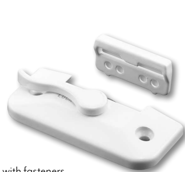
Qty: 1 set, with fasteners. Diecast, 2-1/4 in. hole spacing, cam action, 1/2 in., 3/4 in. and 1 in. keeper hole spacing. F2899 (White)
