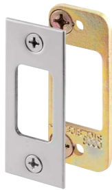
Qty: 1 set, with fasteners. 1/8 in. thick heavy gauge steel base, 2-1/8 in. hole spacing, improves security with 3 in. long screws attaching to wall stud. E 2479 (Brass finish) E 2482 (Bronze finish) E 2480 (Antique brass finish) E 2688 (Stainless steel) E 2483 (Satin nickel finish) E 2796 (Matte black finish)
