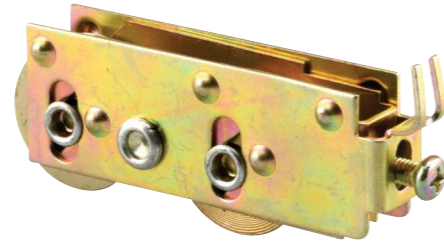
Qty: 1 Steel housing assembly, end adjustable, 1-1/8 in. O.D. tandem steel ball bearing rollers, center grooved.
