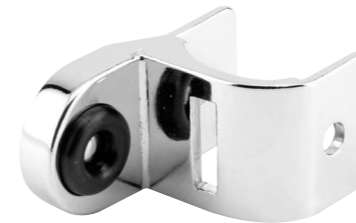
Qty: 1, with fasteners. In/outswing for concealed latch with flat bolt, for 1-1/4 in. thick round edge posts. 656-6533 (Chrome plated zamak)
