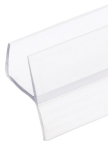
Qty: 1 Clear vinyl, "Y" vertical side seal, 78 in., UV resistant, mold resistant with anti-fungal additives. M 6312 (Fits 1/4 in glass) M 6313 (Fits 3/8 in glass) M 6314 (Fits 1/2 in glass)
