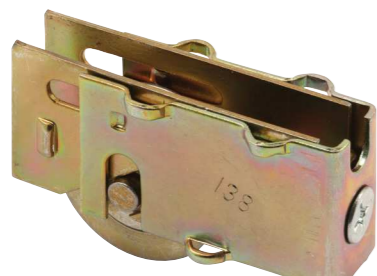
Qty: 1 Steel housing assembly, end adjustable, 1-1/8 in. O.D. steel ball bearing roller, center grooved.
