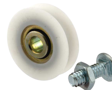
Qty: 2 sets. Plastic ball bearing roller, 1-1/4 in. O.D., 1/4 in. I.D. axle hole, center grooved, with axle carriage bolts and nuts. D 1504
