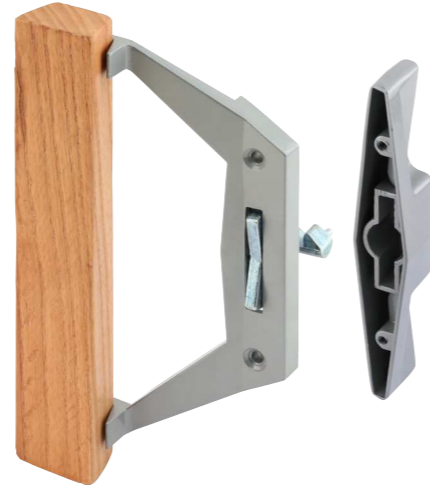
Qty: 1 set, with fasteners. Diecast inside pull with wood handle, diecast outside handle, 3-1/2 in. hole spacing, hook style, internal lock, for Burval® and Trimview®.
