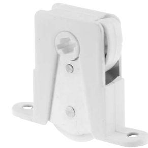
Qty: 2, with fasteners. Aluminum inner housing, plastic outer housing, adjustable, 1 in. O.D. plastic roller, center grooved.
