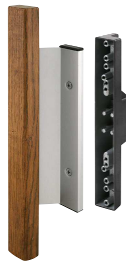
Qty: 1 set, with fasteners. Extruded aluminum inside pull with wood handle and thumbturn, diecast outside handle, 3-15/16 in. hole spacing, hook style, mortise latch, non-handed.
