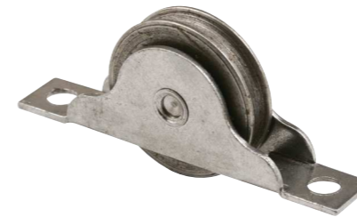
Qty: 2 Steel housing, fits a 2-1/4 in. x 3/8 in. mortise slot, 1-7/8 in. hole spacing, 1 in. O.D. steel ball bearing roller, center grooved.
