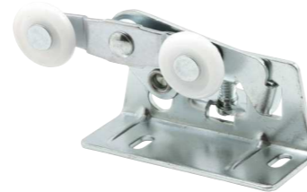
Qty: 2, with fasteners. Steel bracket, top mount, adjustable, tandem 7/8 in. O.D. plastic rollers, round edge, for 1-3/8 in. thick doors.
