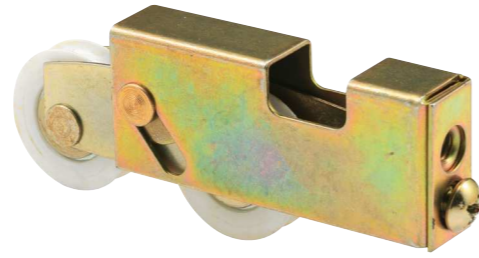
Qty: 1 Steel housing assembly, end adjustable, 1-1/4 in. O.D. tandem ball bearing rollers, center grooved.
