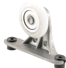
Qty: 1, with fasteners. Steel bracket, top mount, 2-1/4 in. hole spacing, 1-1/4 in. O.D. plastic ball bearing roller, round edge.
