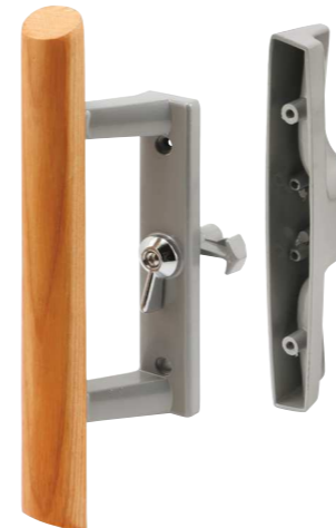
Qty: 1 set, with fasteners. Diecast inside pull with wood handle, diecast outside handle, 3-15/16 in. hole spacing, hook style, internal lock, reversible, for 1 in. thick doors.
