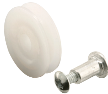
Qty: 2 sets, with fasteners. Plastic roller, 1 in. O.D., 1/4 in. I.D. axle hole, center grooved, machine screw and binder post.
