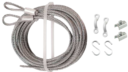
Qty: 2 sets. Galvanized carbon steel, 12 ft. length, 3/32 in. O.D., with cable clamps and hooks. GD 52289
