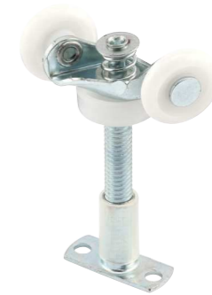
Qty: 1, with fasteners. Steel bracket, top hung, adjustable, tandem 7/8 in. O.D. plastic rollers, round edge, 7/8 in. O.D. plastic guide roller, flat edge, for 3/4 in. to 1-3/8 in. thick doors.
