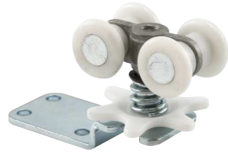
Qty: 1, with fasteners. Steel bracket, spring loaded, adjustable, (4) 23/32 in. O.D. plastic rollers, flat edge, for 1 in. to 1-3/4 in. thick doors.
