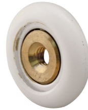
Qty: 2, with fasteners. 3/4 in. O.D. plastic ball bearing roller, round edge, threaded hub, brass inner race.
