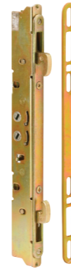
Qty: 1, with fasteners. Steel housing and hooks, round faceplate, multi-point, 45° keyway, 9-7/8 in. hole spacing.
