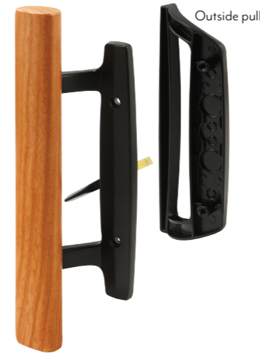
Qty: 1, with fasteners. Diecast inside latch with wood handle and thumbturn, diecast outside handle, 3-15/16 in. hole spacing, hook style, mortise latch, non-handed.
