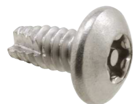
Qty: 100 T-27 pan head, six lobe with center pin, self cutting thread, 3/8 in. length. 642-0118 (Stainless steel)
