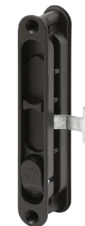
Qty: 1, with fasteners. Diecast inside and outside handles, 5-1/8 in. hole spacing, flush mount hook latch, automatic locking feature.
