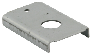
Qty: 2, with fasteners. Steel, used to repair wood doors split at the pivot hole, used with 3/8 in. or 7/16 in. pivots.
