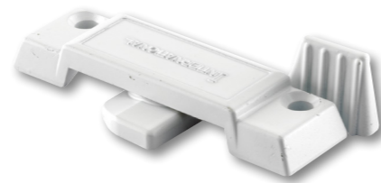
Qty: 1, with fasteners. Diecast, 2-1/4 in. hole spacing, cam action, used on International Windows®. F2780 (White)
