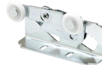
Qty: 2, with fasteners. Steel bracket, top mount, adjustable, tandem 7/8 in. O.D. plastic rollers, round edge, for 3/4 in. to 1-3/8 in. thick doors.
