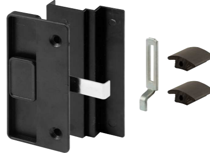
Qty: 1, with fasteners. Plastic inside and outside handles, steel latch, steel keeper, vinyl guides, 3 in. hole spacing, non-handed.
