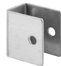
Qty: 1, with fasteners. "U" bracket, stamped stainless steel, 14 gauge, 1-1/2 in. length.
