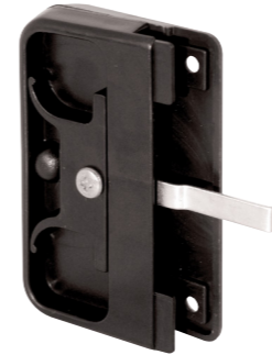
Qty: 1, with fasteners. Plastic inside and outside handles, steel latch, 2-5/8 in. hole spacing, non-handed.
