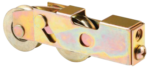
Qty: 1 Steel housing assembly, end adjustable, 1-1/4 in. O.D. tandem steel ball bearing rollers, center grooved.
