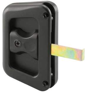
Qty: 1, with fasteners. Plastic inside and outside handles, steel latch, 3 in. hole spacing, non-handed, for "Hat Section" style doors.
