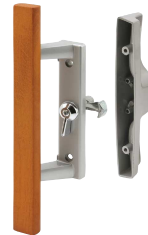
Qty: 1 set, 2 keys, with fasteners. Diecast inside pull with wood handle, diecast outside handle, 3-15/16 in. hole spacing, hook style, internal lock, reversible, keyed, for 1 in. thick doors.
