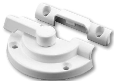
Qty: 1 set, with fasteners. Diecast, 1-7/8 in. hole spacing, cam action, keeper has 2 in. hole spacing. F2918 (White)
