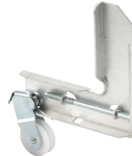
Qty: 1 Stamped steel housing, adjustable, 1 in. x 11/32 in. leg, 15/16 in. O.D. plastic roller, center grooved.
