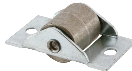
Qty: 2 Steel housing, fits a 1 in. groove, 1-9/16 in. hole spacing, 3/4 in. O.D. steel roller, flat edge.
