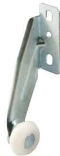
Qty: 2, with fasteners. Steel bracket, right hand (determined as viewed from rear of drawer), convex plastic roller, 13/16 in. O.D., mounts on rear of drawer.
