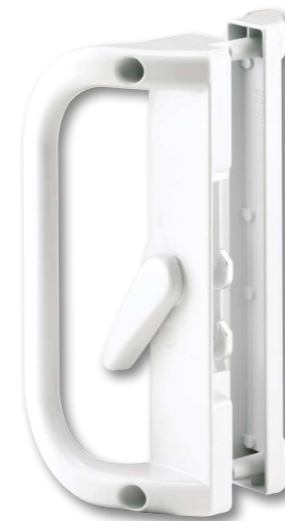
Qty: 1 set, with fasteners. Diecast aluminum handles, 6-9/16 in. hole spacing, dual hook style latch, surface mounted, primarily used in Canada.
