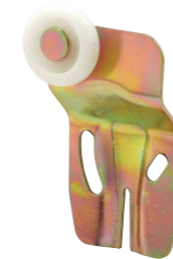
Steel bracket, top hung, adjustable, 7/8 in. O.D. plastic roller, round edge, for 3/4 in. to 1-3/8 in. thick doors.
