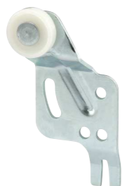
Qty: 2, with fasteners. Steel bracket, top hung, adjustable, 3/4 in. O.D. plastic roller, flat edge, for 3/4 in. to 1-3/8 in. thick doors.
