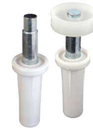
Qty: 1 set. Top mount, 7/16 in. O.D. plastic base, spring loaded, self-adjusting, 7/8 in. O.D. plastic roller, flat edge, 1/4 in. O.D. steel tip, for 1 in. to 1-3/8 in. thick doors.
