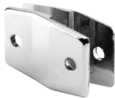
Qty: 1 set. Joins laminate panel to pilaster, 1/8 in. offset per clip, 1-1/2 in. hole spacing. 650-6656 (Chrome plated zamak, no fasteners ) 656-6656 (Chrome plated zamak, with fasteners ) 656-6656-T (Chrome plated zamak, with T-27 fasteners ) 656-4028 (Satin cast stainless steel, with fasteners ) 656-4028-T (Satin cast stainless steel, with T-27 fasteners )
