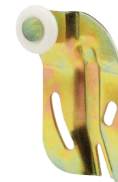
Steel bracket, top hung, adjustable, 3/4 in. O.D. plastic roller, round edge, for 3/4 in. to 1-3/8 in. thick doors.
