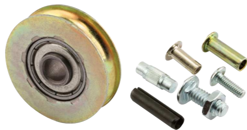
Qty: 2 sets. Ball bearing roller, 1/4 in. I.D. axle hole, center grooved, with axle pins, roll pins, rivets, binder posts, axle carriage bolts and nuts. D 1795 (1-1/8 in. O.D. - Steel) D 1799 (1-1/2 in. O.D. - Plastic) D 1798 (1-1/4 in. O.D. - Plastic) D 1797 (1-1/2 in. O.D. - Steel) D 1796 (1-1/4 in. O.D. - Steel)
