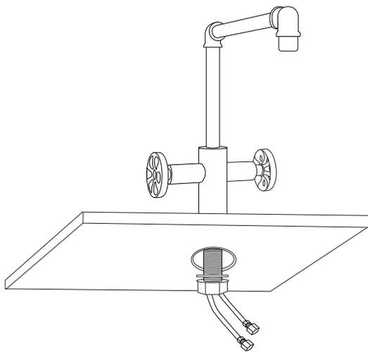
3. From beneath the sink, slide the rubber washer back onto the faucet body. Thread the locknut back onto the shank until hand tight. Finish tightening using a basin wrench.
