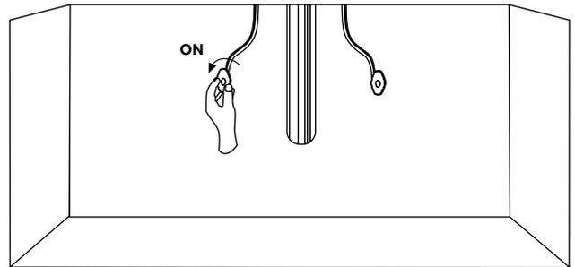
9. Turn the faucet on and ensure that there are no leaks. Check to ensure that both hot and cold water are running properly. Allow the water to flow for approximately 60 seconds to remove any dust or sediment within the water lines.
