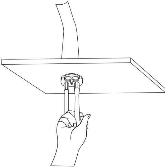
7. Apply plumber's tape or thread sealant to the threading on each braided water line. Attach the water lines to your main water supply lines. Ensure that you are connecting the hot and cold lines appropriately.
