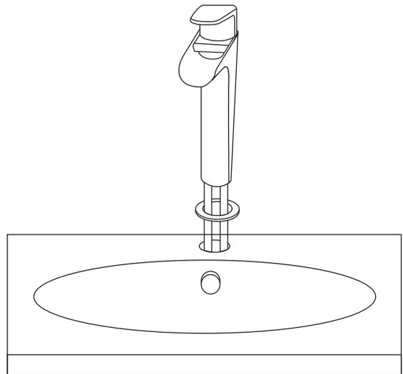
5. From beneath the sink, slide the rubber gasket onto the mounting posts, followed by the metal washer. Ensure that each post passes through its designated hole. Hold in place.
