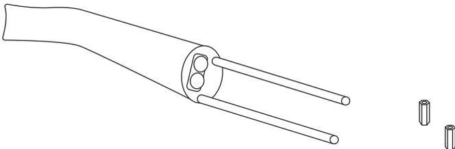
4. Slide the decorative escutcheon onto the braided water lines and up to the faucet body. From above the counter top, set the faucet into its prepared mounting hole.
