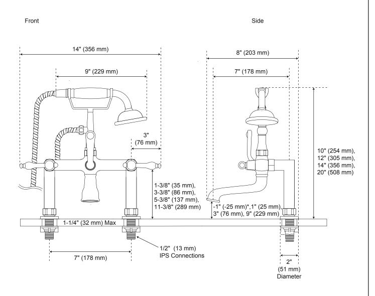
\*Faucet spout extends below deck when installed with 2" couplers.
