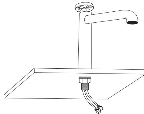
4. Apply plumber's tape or thread sealant to the threading on each of the faucet's water lines, and connect the main water hoses to the faucet. Use an adjustable wrench to tighten, but be careful not to overtighten. Ensure that you are connecting the hot and cold lines appropriately.
