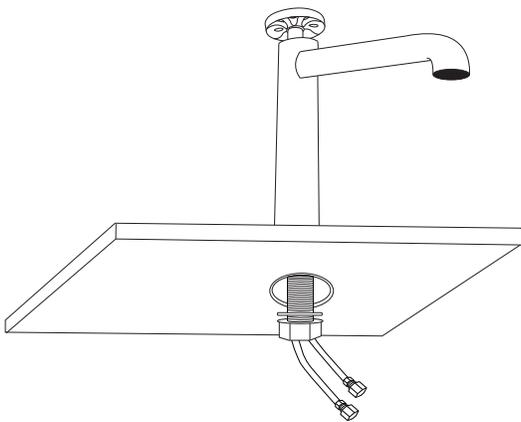
3. From beneath the sink, slide the rubber washer back onto the faucet body. Thread the locknut back onto the shank until hand tight. Finish tightening using a basin wrench.
