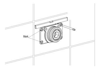
4. Use a level to ensure that the base is aligned properly, and mark the locations of the mounting holes.
