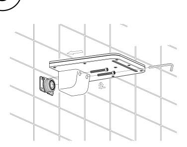
8. Attach the faucet body to the base with M5 screws.
