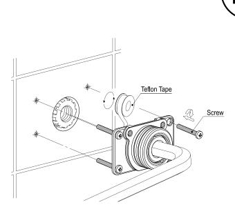
7. Wrap teflon tape around the threaded pipe on the base. Screw the base into the water outlet, and drive screws the through base into the wall anchors.
