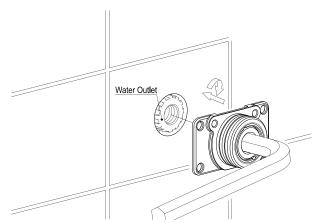
3. Screw the base into the fitting with the provided 12mm hex wrench.
