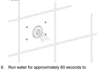
6. Run water for approximately 60 seconds to remove dirt and debris from the pipe.
