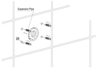
5. Remove the base and drill mounting holes in the locations marked in the previous step. Insert wall anchors into the mounting holes.
