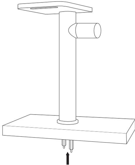
6. Apply plumber's tape or thread sealant to the threading on each braided water line. Attach the water lines to your main water supply lines. Ensure that you are connecting the hot and cold lines appropriately.
