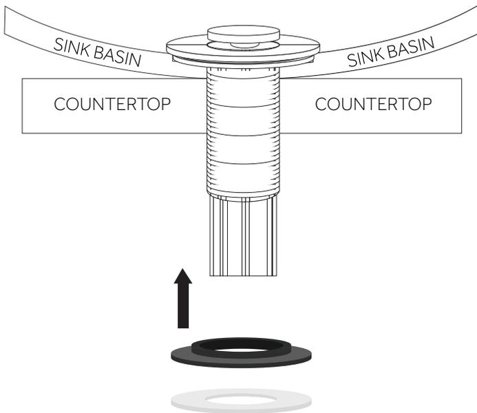
6. Thread the lock nut onto the drain flange. Hand tighten until secure, then finish tightening with a basin wrench once the drain is properly aligned.
