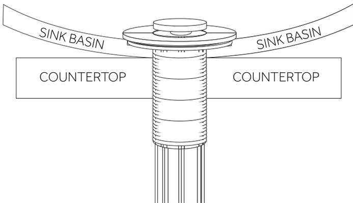
5. From under your counter, slide the tapered rubber gasket followed by the plastic friction washer onto the tailpiece until they meet your sink or countertop. Be sure that the tapered side of the rubber washer is facing up.
