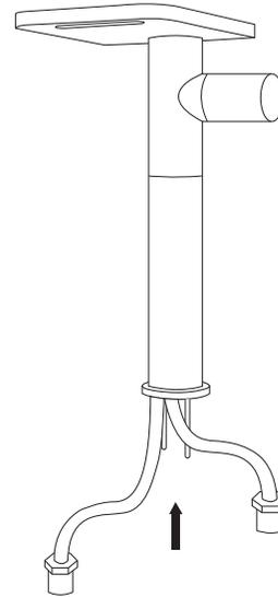
4. Insert the faucet into the mounting hole. From beneath the sink, slide the rubber gasket onto the mounting posts followed by the metal washer. Ensure that each post passes through its designated hole. Hold in place.
