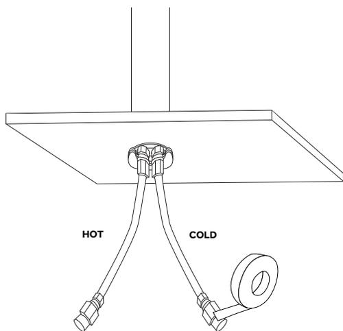
7. Once installation is complete, turn the main water supply back on from underneath your sink. Check for any leaks underneath.
