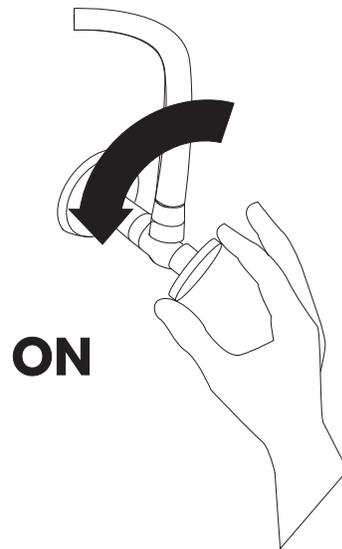
8. Proceed to drain installation. Once complete, turn the faucet on. Check for leaks. Check to ensure that both hot and cold water are running properly. Allow the water to flow for approximately 60 seconds.
