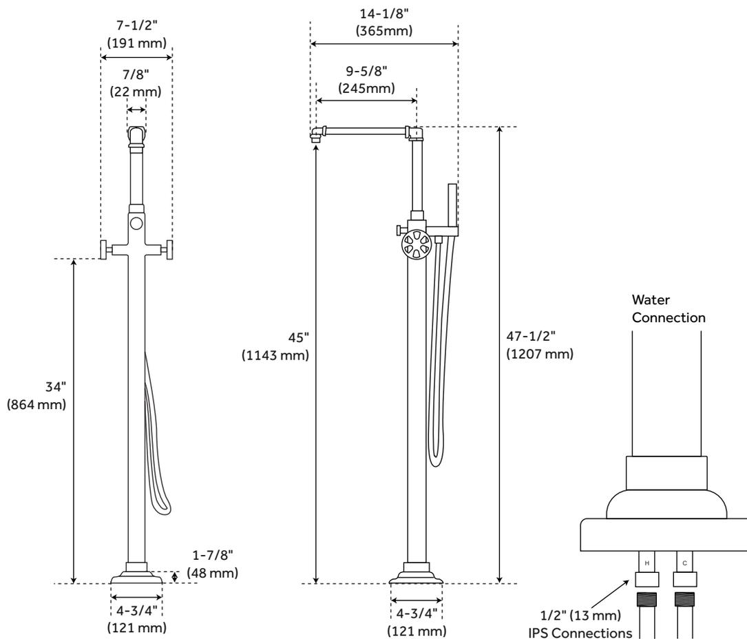
Underfloor access is required for proper installation.
