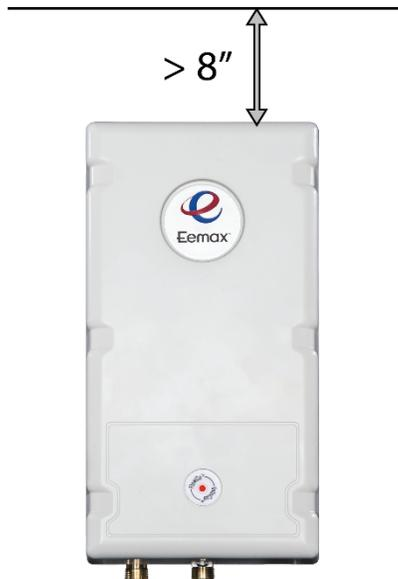
**3.** Remove the cover and fasten to the wall using the four mounting holes at each corner of the back plate. Replace the cover.
