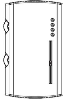
Auto, Heat, Cool or Off System Switch. Fan Auto or Off Switch. Two temperature setpoint levers. Status Indication LED lights, System On, Heat, Cool, or Service.
