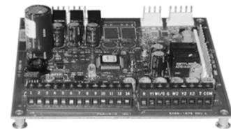
Voyager with ReliaTel reduces the number of components required to operate the unit, thereby reducing possibilities for component failure.
