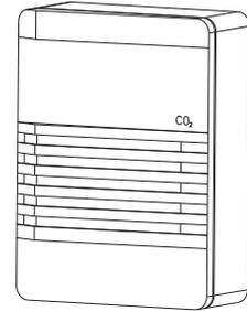
The CO<sub>2</sub> sensor shall have the ability to monitor the concentration (parts per million, ppm) of CO<sub>2</sub> (Carbon Dioxide) in the air. As the CO<sub>2</sub> concentration changes, the outside air damper modulates to meet the current ventilation needs of the zone.
