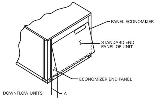
**Note:** When applying economizer to horizontal units, connected ductwork must be run full size to allow proper operation of economizer damper.
