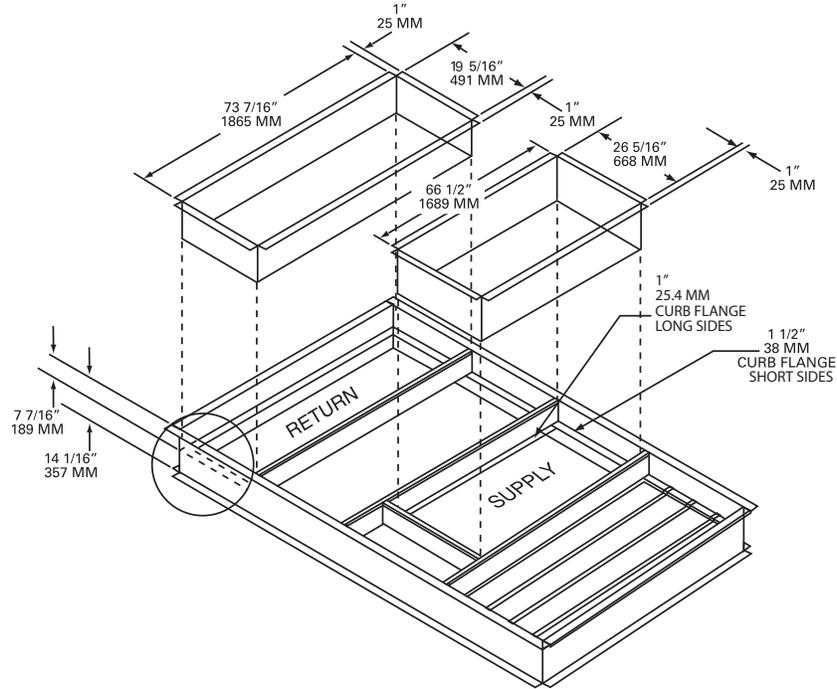
\* Duct flanges mount 7-7/16" down inside the curb on the 1-1½ curb flanges.
