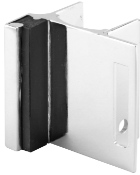
Qty: 1, with fasteners. Inswing for slide latch, for 1-1/4 in. thick round edge posts, 1-1/2 in. hole spacing. 656-6515 (Chrome plated zamak)
