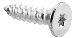
Qty: 100 T-20 flat head, six lobe with center pin, #10 x 1 in. 645-0140 (Chrome) 642-0140 (Stainless steel)
