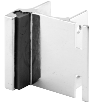
Qty: 1, with fasteners. Inswing for throw latch (emergency entrance), for 1-1/4 in. thick round edge posts, 1-1/2 in. hole spacing. 656-6521 (Chrome plated zamak)
