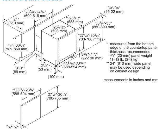
\* thickness recommended <sup>3</sup>/4" (20 mm), panel weight 11–18 lb. (5–8 kg)
