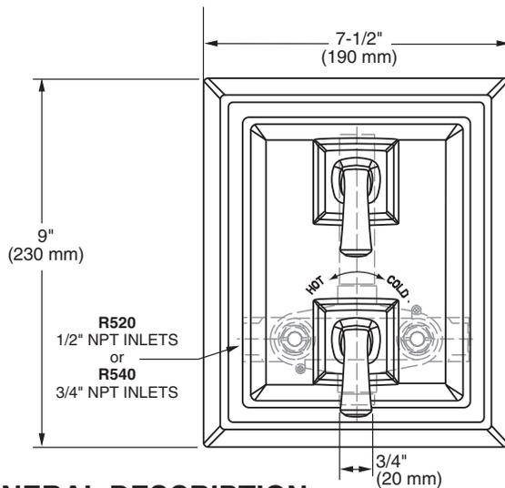
NOTE: FITTING MUST BE INSTALLED WITH VOLUME CONTROL ON TOP.
