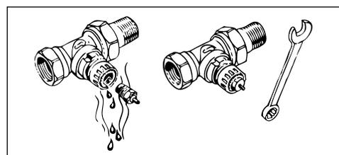
Should the packing gland on the valve body show signs of weeping, it can be replaced in a few minutes with the system in operation.
