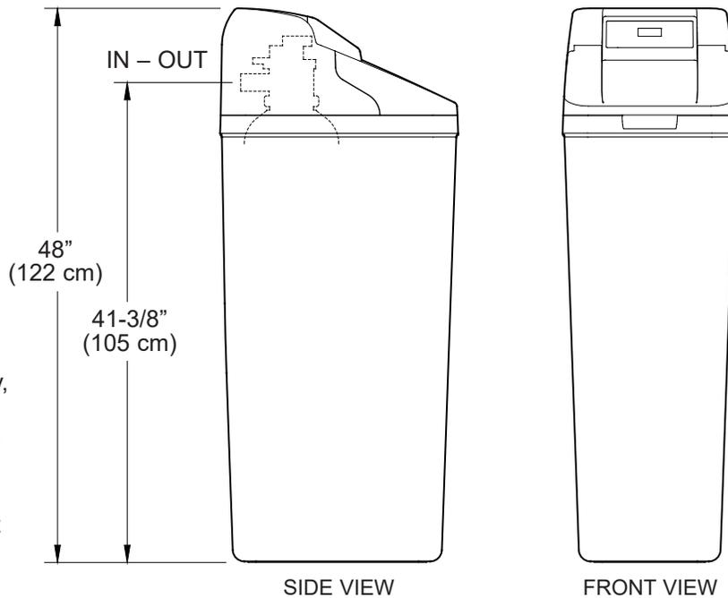
**NOTE:** Due to variances in production and assembly, the water softener valve height may vary by up to 1/2", and may not match previously installed systems. This will not affect system performance.
