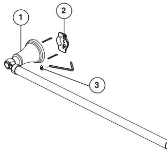
Position body (1) over mounting bracket (2) and tighten set screw (3). (Set screw should be on the bottom of body.) Place one end of the towel bar (4) into the second body (5), and place the other end of the bar into the first body (1). Slide the second body over the other mounting bracket (6) and tighten set screw (7).
