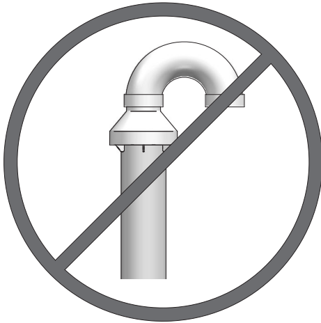
Figure 5-5 Do Not Install U-Bend to Rain Cap
