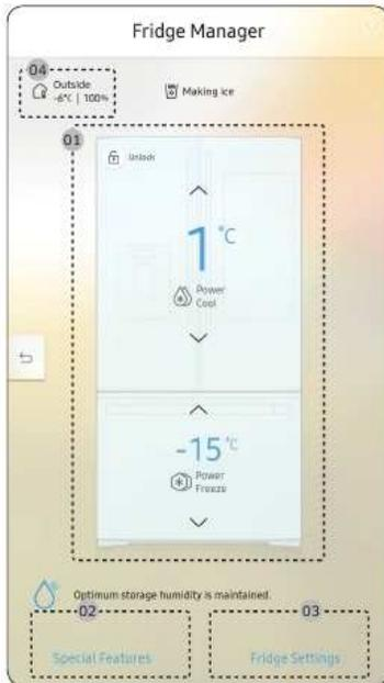
The Fridge Manager is a graphical representation of your refrigerator. The top half represents the refrigerator compartment, and the bottom half represents the freezer compartment. The temperature or mode settings for each are displayed over each section.
