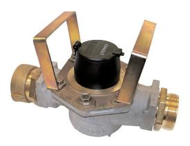
The HT4000 is intended for use with fire hydrants for temporary measurement of potable cold water (up to  $120 \, ^{\circ}\text{F} / 50 \, ^{\circ}\text{C}$ ) up to  $150 \, ^{\circ}\text{PSI}$ , for use on construction sites and similar locations.
