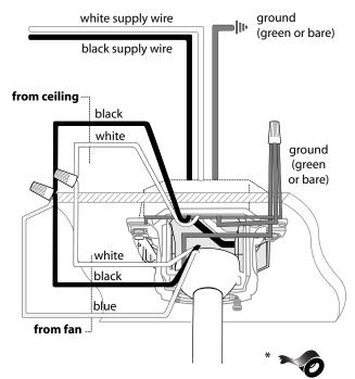
\* Wrap each wire connector separately with electrical tape as an extra safety measure.
