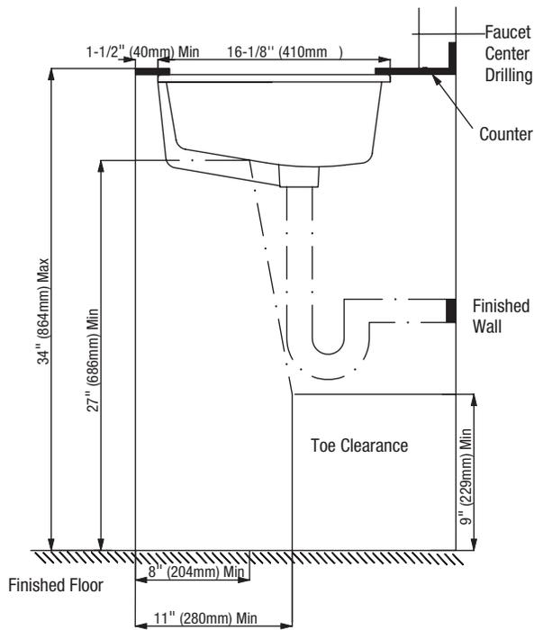
\*All dimensions and specifications are nominal and may vary: Dimensions of 8" and greater have a tolerance of +3%. Dimensions less than 8" have a tolerance of +5%. Please utilize the current cutout template for countertop cutouts.
