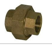
A.Y. M<sup>o</sup>Donald Mfg. Co. No-Lead Pipe Fittings & Nipples are constructed from heavy duty bronze and are rated for commerical, industrial and residential applications up to 125 WOG. Threads conform to ANSI B1.20.1 and fitting dimensions comply with ANSI B16.15.
