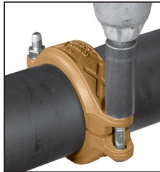
**7 ASSEMBLY IS COMPLETE** Visually inspect the pipe joint to assure the coupling keys are fully engaged in the pipe grooves. The bolt pads are to have equal gaps on each side of the coupling.
