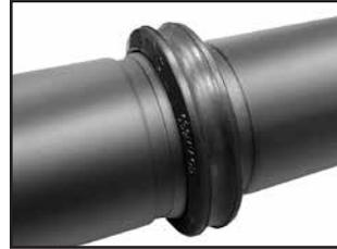
**4 PIPE ALIGNMENT AND GASKET INSTALLATION** Slide the gasket onto the pipe then align the two pipe ends together. Pull the gasket into position, centering it between the grooves on each pipe. Gasket should not extend into the groove on either pipe.
