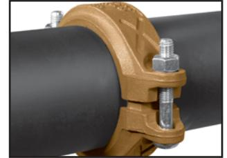
**5 HOUSING ASSEMBLY** Place each housing halves on the pipe making sure the housing key fits into the groove. Be sure that the tongue and recess portions of the housing mate properly. Insert the bolts.
