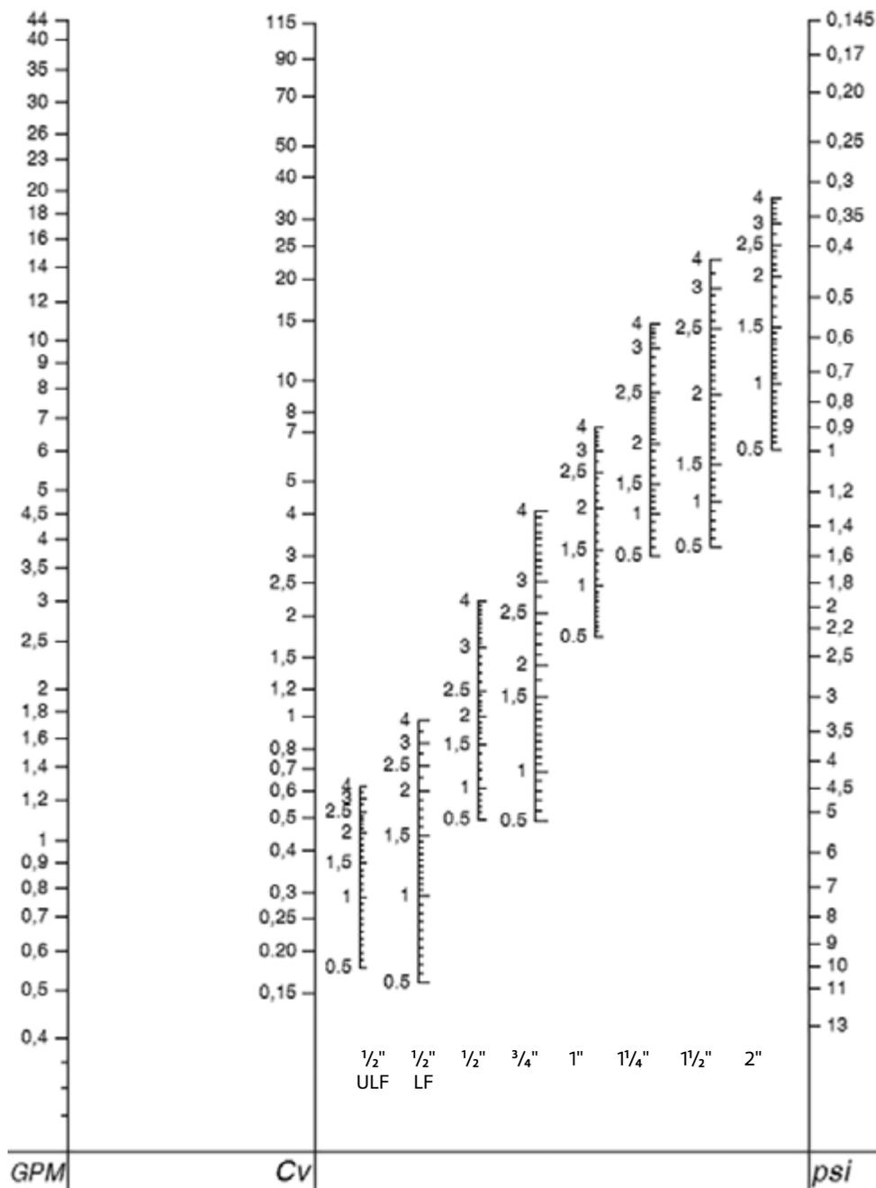
Using diagram above, determine the presetting position of the valve with the given design flowrate and headloss:
