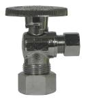
A.Y. McDonald Mfg. Co. No-Lead Quarter Turn Supply Stops are fully certified to all applicable standards. The Ball Valve design allows for ease of operation and positive shut-off and is ideal for residential and commercial applications. Each valve is constructed of heavy duty chrome plated brass.
