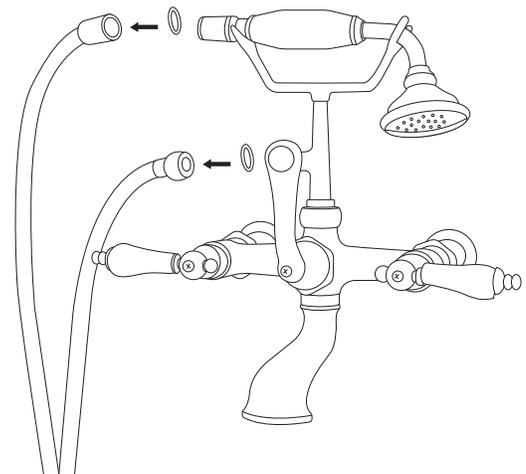
10. Turn on the main water supply, then turn the faucet on. Allow the water to flow for approximately 60 seconds. Divert the water to the hand shower and allow the water to flow for another 60 seconds. Check to make sure that all connections are tight, and there are no leaks.
