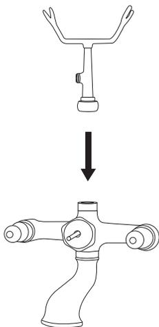
9. Attach the hand shower to the faucet by using the provided flexible hose. Connect the hose to the outlet located on the cradle. Place the hand-held shower in the cradle.
