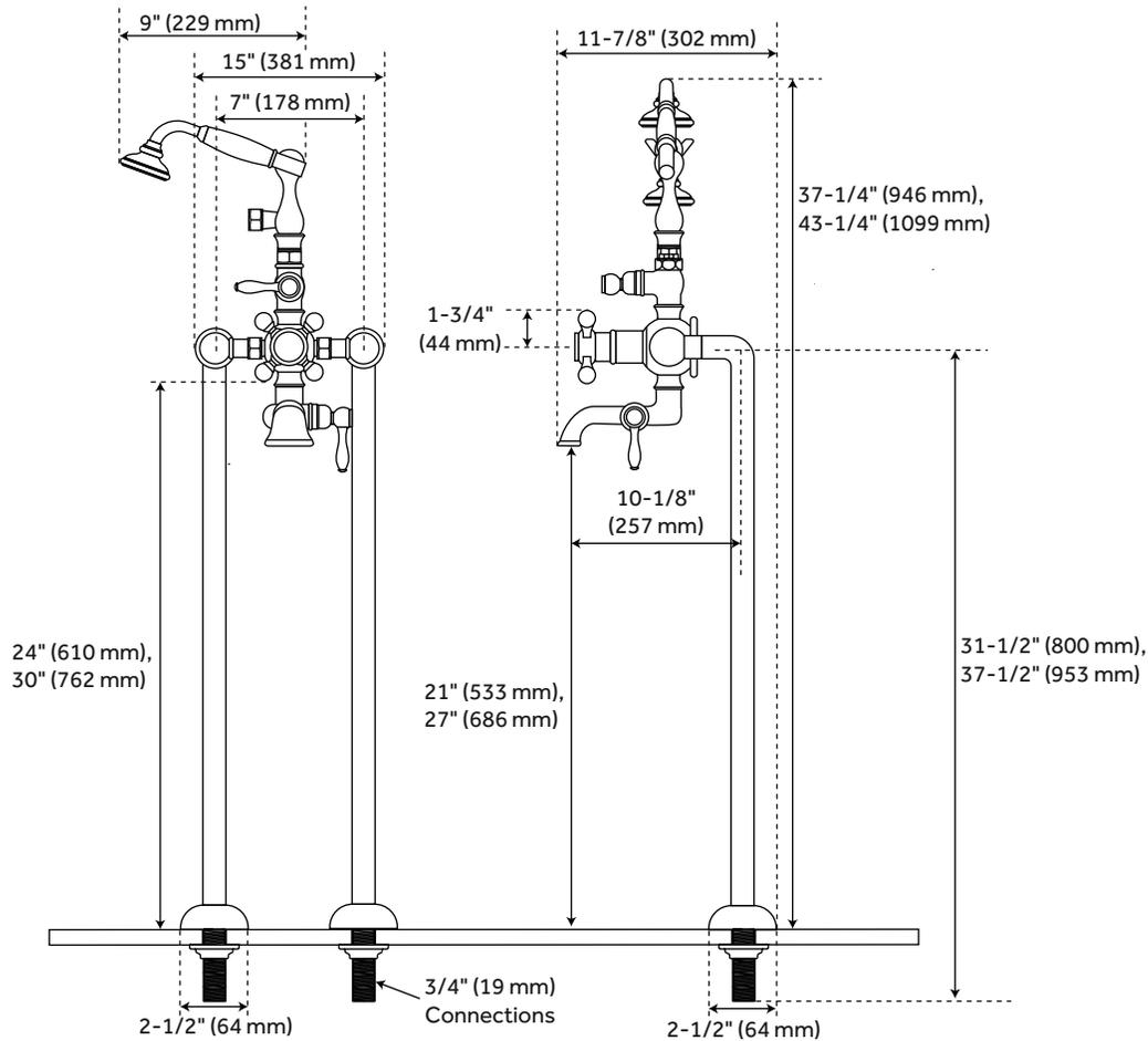
Underfloor access is required for proper installation.
