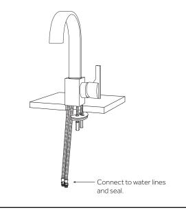
5. Once installation is complete, turn the main water supply back on from underneath your sink. Check for any leaks underneath.
