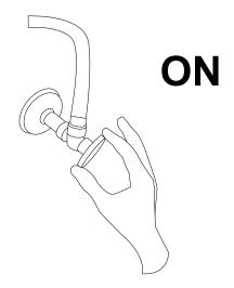
6. Turn the faucet on for approximately 60 seconds to check for any leaks. Ensure that both hot and cold water are functioning properly.
