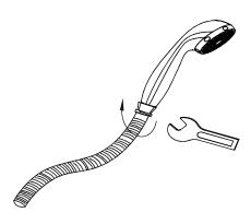
2. Install new handshower on the hose. Thread the hose nut onto the handshower clockwise.
