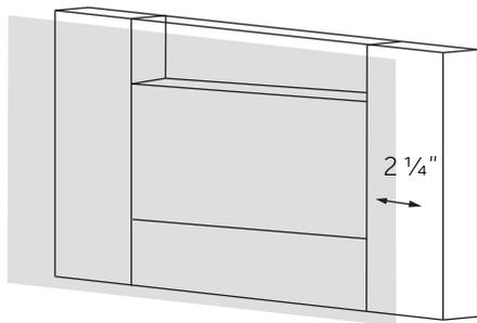
2. Secure the valve to the prepared wood blocking using the provided hardware. Ensure that the "cold" inlet is pointing to the right, and the "hot" inlet is pointing to the left. Use a level to ensure that the valve is straight and level. Leave the protective sleeves on the valve stems until your finished wall is complete, and you are ready to install the trim pieces.
