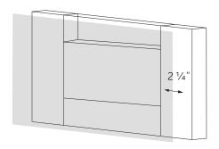
2. Secure the valve to the prepared wood blocking using the provided hardware. Ensure that the "cold" inlet is pointing to the right, and the "hot" inlet is pointing to the left. Use a level to ensure that the valve is straight and level.
