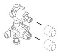
2. Slide the decorative back plate onto the valve. Ensure that the markings located above each opening on the back plate are facing up. Install the handles using the provided hex wrench.
