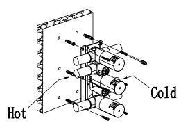
Install the valve body. Wrap the threaded portion of the joints in Teflon tape and connect the water inlet and outlet.
