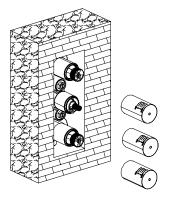
3. When the finished wall is complete, remove the protective covers.
