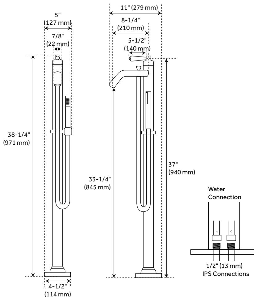
Underfloor access is required for proper installation.
