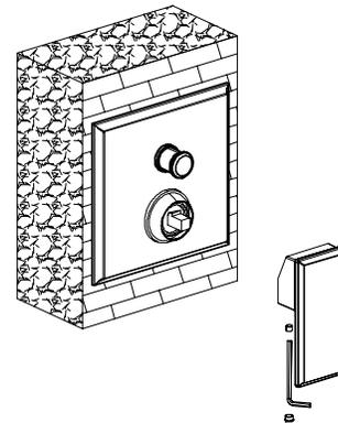
4. Install the escutcheon, and handle. Tighten the set screw with an Allen wrench to secure.
