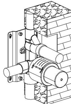
2. Put the protective covers on the valve body and finish the shower wall.
