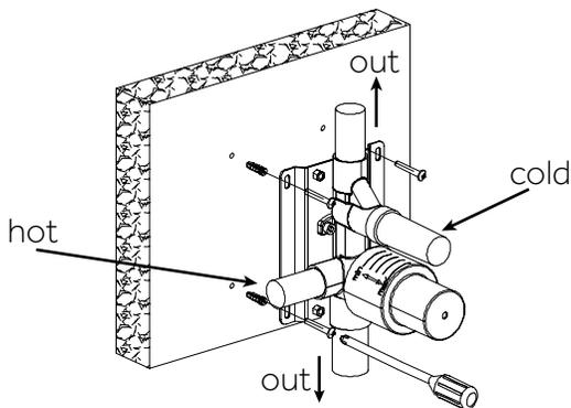
1. Install the valve body. Wrap the threaded portion of the joints in Teflon tape and connect the water inlet and outlet.
