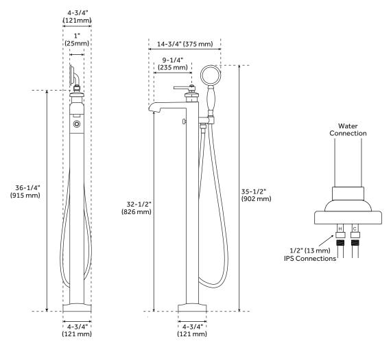
$\label{thm:condition} Underfloor\ access is\ required\ for\ proper\ installation.$  Installation on a concrete slab will require cutting and concrete removal.
