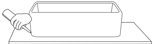
4. Remove any excess sealant with a damp cloth to complete installation.
