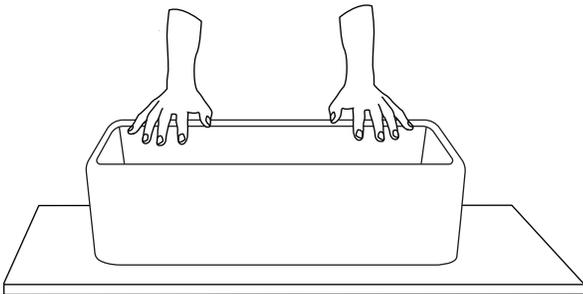
3. If desired, apply a continuous bead of silicone sealant around the perimeter of the sink base for additional stability.
