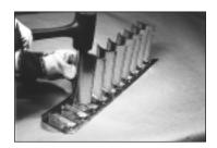
4. Insert the top rail tabs into the vanes.
