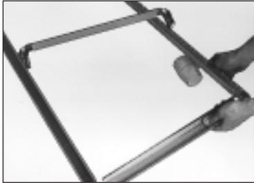
4. Slide two longer angle pieces onto corner pieces already inserted into shorter pieces, then add the second short piece to complete the frame.
