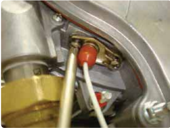
Figure 138 Removal of Ignition electrode
