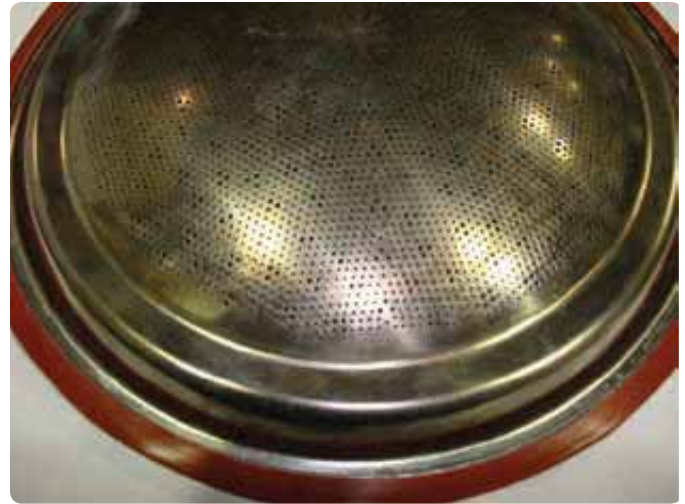
Figure 144 Inspecting exterior and cleaning the burner
