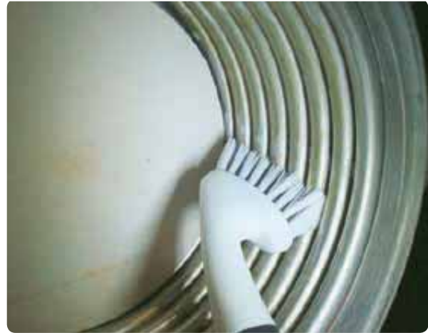
Figure 147 Cleaning the heat exchanger
