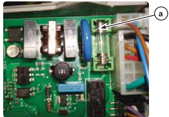
Figure 116 Thermostat-relay circuit fuse location
