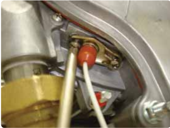
Figure 142 Removal of Ignition electrode
