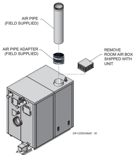
The XP Plus uses model specific combustion air intake and vent piping sizes as detailed in Tables 3B and 3C on page 18.
