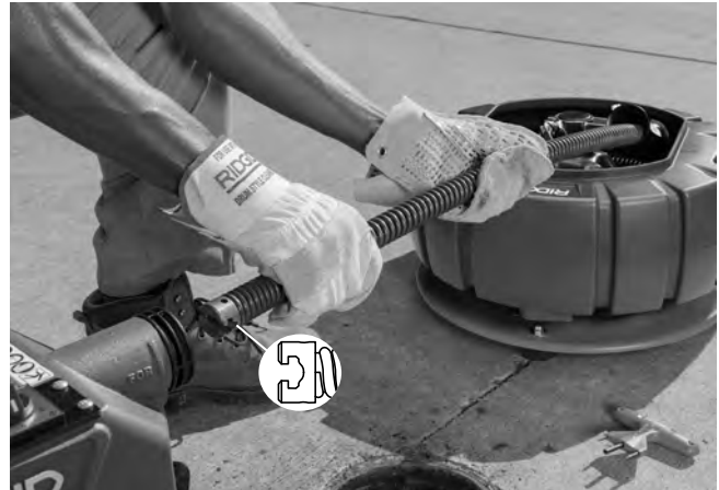
Figure 7 – Inserting Cable Into Front Of Machine
