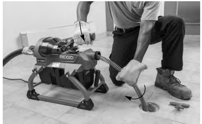
Figure 11A – Clutch Engaged, Cable Rotating, Feeding Cable Into Drain
