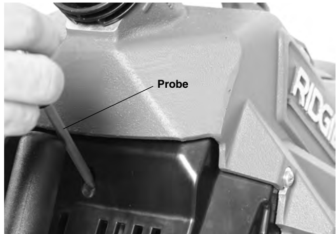
Figure 22 – Motor Reset Button
