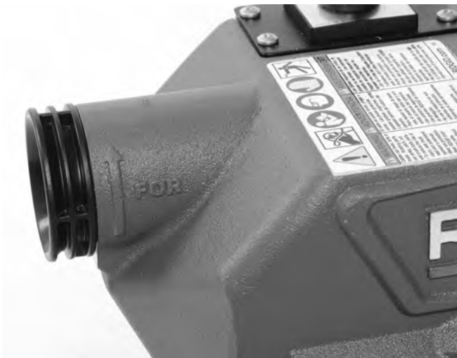
Figure 10 – FOR Machine Rotation Marking
