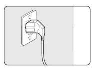
Plug the power cord into a 3-prong, well grounded 120 volt 60 Hz approved electrical outlet protected by a 15-amp fuse or comparable circuit breaker.
