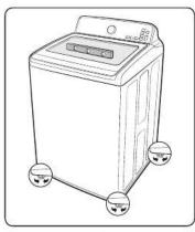
If the washer is level, the pulsator (A) is positioned at the center of the water as shown in the figure.
