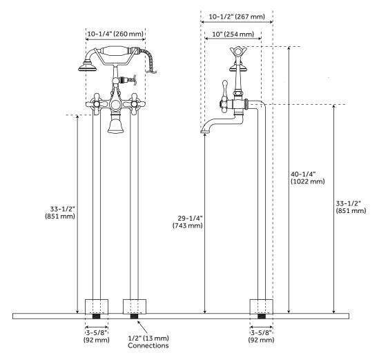
$\label{thm:condition} Underfloor\ access is\ required\ for\ proper\ installation.$  Installation on a concrete slab will require cutting and concrete removal.
