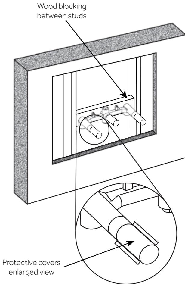
2. Mount the rough-in valve into its prepared location. Attach the valve body using the provided hardware. Use a level to ensure that the valve is mounted completely level.
