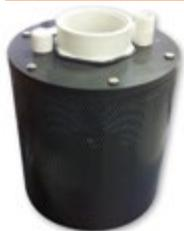
The simple operation of this device makes it a good all around strainer. A small amount of water is returned from the pressure side of the pump to the strainer. Inside, two nozzles spray the screen off and any debris attached to the screen will be removed.
