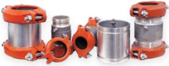
The Munro grooved check valve features an aluminum or brass body and a Buna-S spring assisted tapered style poppet. This design lends itself to low flow or pulsating flows to reduce cavitation and chattering. This valve was designed with irrigation systems in mind. All internal Parts are rubber or stainless steel.
