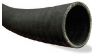
Rubber Water Suction Hose is a general-duty service hose. This hose offers a long life and increased bend radius when compared to general purpose PVC hose. Temperature -40° – 180° F
