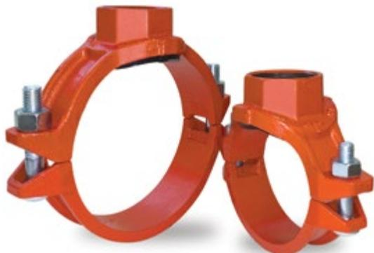
Outlet couplings, sometimes called mechanical tee or saddle tee, allow you to create a mid-pipe branch outlet quickly and easily. A gasket seals on the joined pipe, in the neck of the outlet. The connection is female threaded. These fittings are not recommended for vacuum applications.
