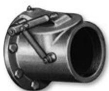
Cast iron discharge valve bolts directly to pump for priming and pump protection. The valve comes with automatic, spring activated mechanism with external handle.
