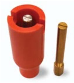
Wire suspension electrodes are designed for use in applications requiring long lengths, or where limited head room prevents installation of solid rod electrodes. Type E-1P shielded electrode is assembled in a molded plastic insulating shield 7/16" in diameter. Type E-1S shielded electrode is assembled in a molded plastic shield 9/16" in diameter.
