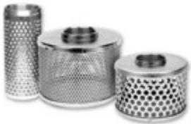
Basket Strainers can be used with all makes of centrifugal pumps. An "open" area of 50% allows strainers to filter out large damaging debris, yet permits sufficient water passage to keep pumps functioning at full capacity.
