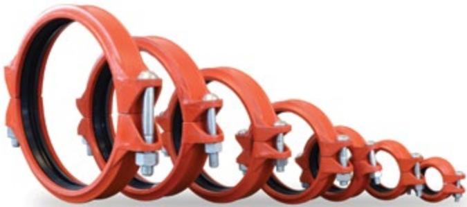
Made to USA standards, to easily interchange with other major manufacturers, the Munro flexible coupling is ideal for use in countless piping applications where misalignment might be present. The M7705 can accommodate vibration, thermal stress and moderate seismic activity. This tried and true coupling offers pressure ratings to 500 PSI, depending on pipe size and wall thickness.
