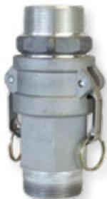
Use this simple fitting assembly facing either direction, both parts will fit into the pump inlet. Quick cams transition from pump inlet to isolation valve on suction piping for easier installation and maintenance of your suction line. Perfect for use in our Universal PRO Pump Enclosure, or anywhere you desire easy connect and disconnect access on the suction side of your pump.
