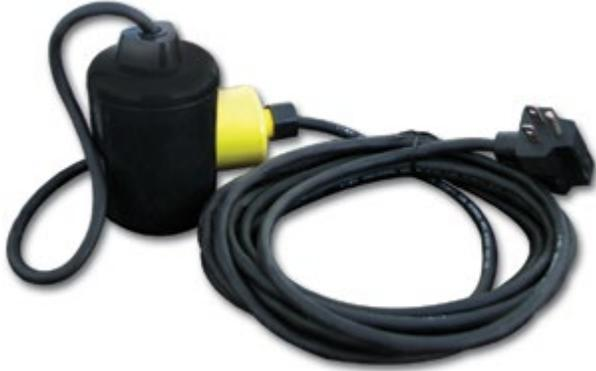
The Munro FloatControl is a direct acting, in-line control system for automatically controlling 1/2 hp and smaller pump motors, or used in conjunction with a pump start relay to accommodate larger hp motors.
