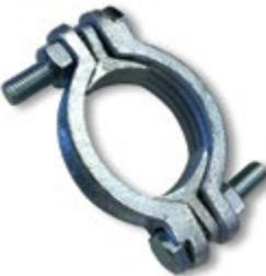
These reusable clamps provide an efficient means to secure fittings for larger size, light or heavy wall hoses. Two-bolt design provides quadruple, full-circumference take-up. Double-tongue saddles bridge the gap between the reinforced, full-width bolt lugs as clamp is tightened, preventing pinching the hose. Can be attached in field or factory with standard tools. Manufactured with plated malleable iron, with steel machine bolts and nuts.
