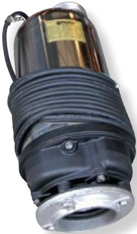
This amphibious pump designed for continuous duty water features does not need a vault. The pump can be positioned at the bank instead of the bottom of a non-potable water source because a hose and strainer allows remote intake of fluid. RP amphibious pumps can also be piped pump to pump to double the pressure!
