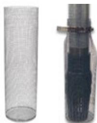
Munro strainers are made of galvanized 1/8" hardware cloth for suction screening and may be easily folded and clamped to pipe.
