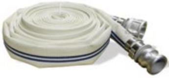
Mill Hose is a single jacket lightweight 150 PSI hose designed for clean-up and wash-down in factories and yards. An ideal industrial discharge hose. Polyester reinforces an ozone-resistant extruded synthetic rubber tube. Temperature -58° – 150° F
