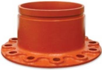
This all-in-one universal flange adapter accepts ANSI 125/150, PN10, PN16, JIS, 10K and BS-10E flange patterns. In addition, a longer grooved end makes this unique fitting easier to install.
