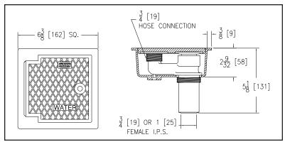
ENGINEERING SPECIFICATION: ZURN Z1375 Encased, moderate climate ground hydrant for flush with grade or finished floor installation. Complete with all bronze interior parts, replaceable bronze seat and seat washer, and non-turning operating coupling with free-floating compression closure valve. D.C.C.I. box and scoriated hinged cover with "WATER" cast on cover.
